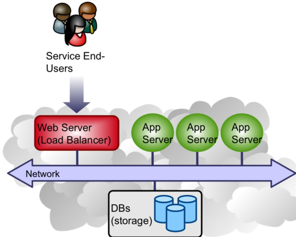
An OpenNebula Private Cloud provides infrastructure users with an **elastic platform for fast delivery and scalability of services to meet dynamic demands of service end-users**. Services are hosted in VMs, and then submitted, monitored and controlled in the Cloud by using *Sunstone* or any of the OpenNebula interfaces:
