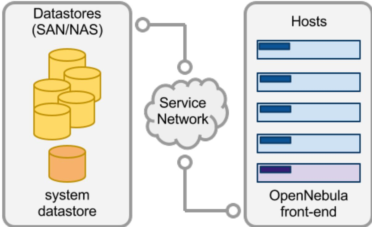
When a VM is deployed the Images are *transferred* from the Datastore to the hosts. Depending on the actual storage technology used it can mean a real transfer, a symbolic link or setting up an LVM volume.
