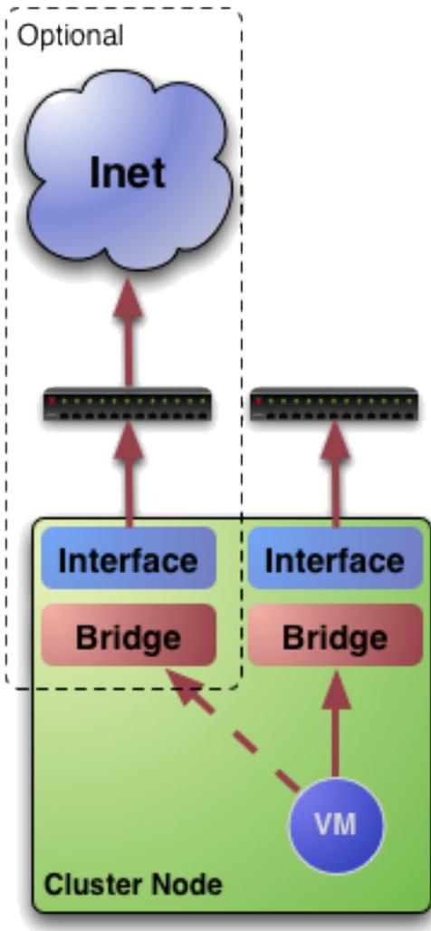
A network connection is needed by the OpenNebula front-end daemons to access the hosts to manage and monitor the hypervisors; and move image files. It is highly recommended to install a dedicated network for this purpose.
