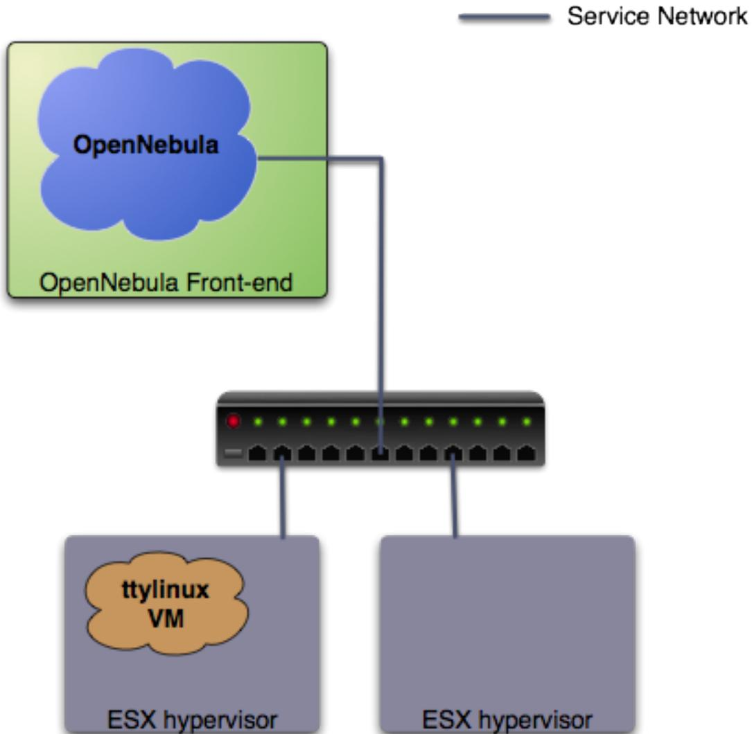
In this guide it is assumed that at least two physical servers are available, one to host the OpenNebula front-end and one to be used as a ESX virtualization node (this is the one you need to configure in the following section). The figure depicts one more ESX host, to show that the pilot cloud is ready to grow just by adding more virtualization nodes.
